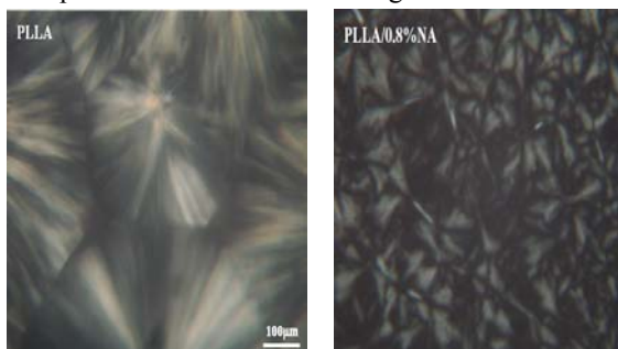
Fig. 4: POM images of PLLA and PLLA/0.8%NA at 115°C.
